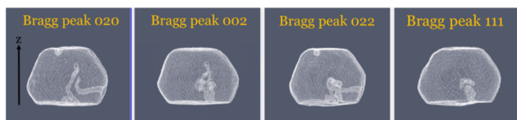
Figure 2: Semi-transparent reconstructions of multi-Bragg reflections after indentation showing the characteristic induced defects for each Bragg peak. (CRISTAL-SOLEIL)
